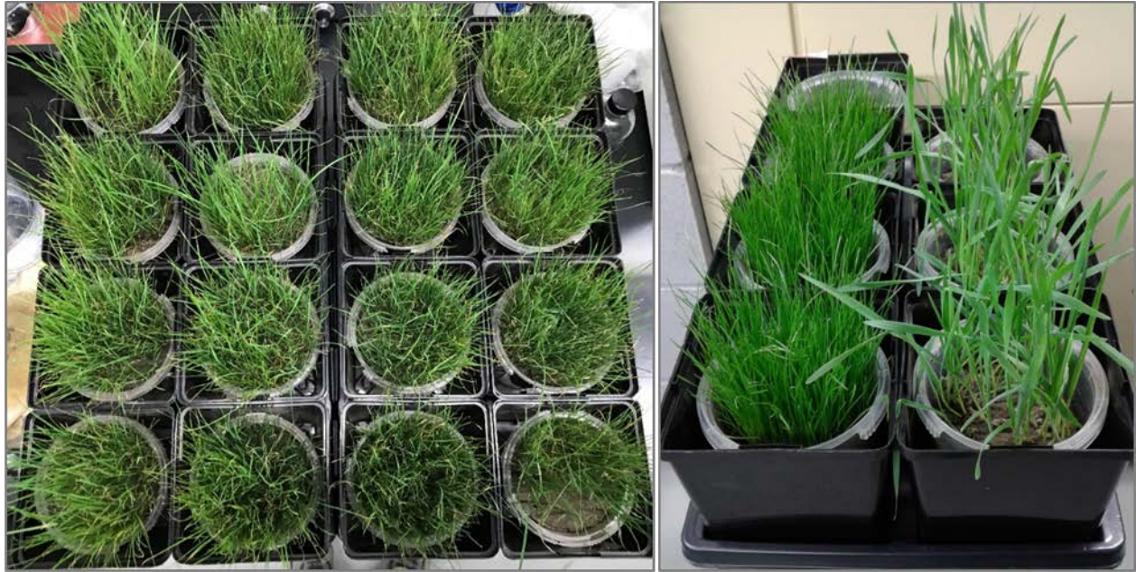
Figure 2. PEPSystems growth trials using soil collected from a contaminated site (left) and control soil spiked with a contaminant (right).
