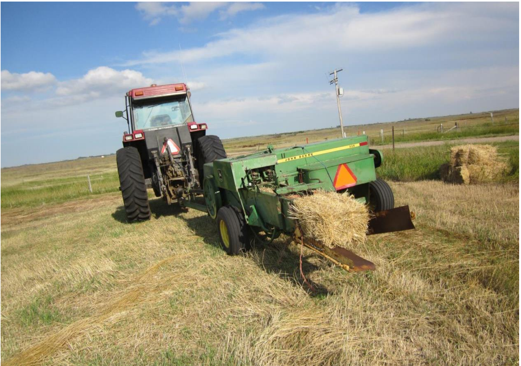
Baling vegetation for removal from site.
